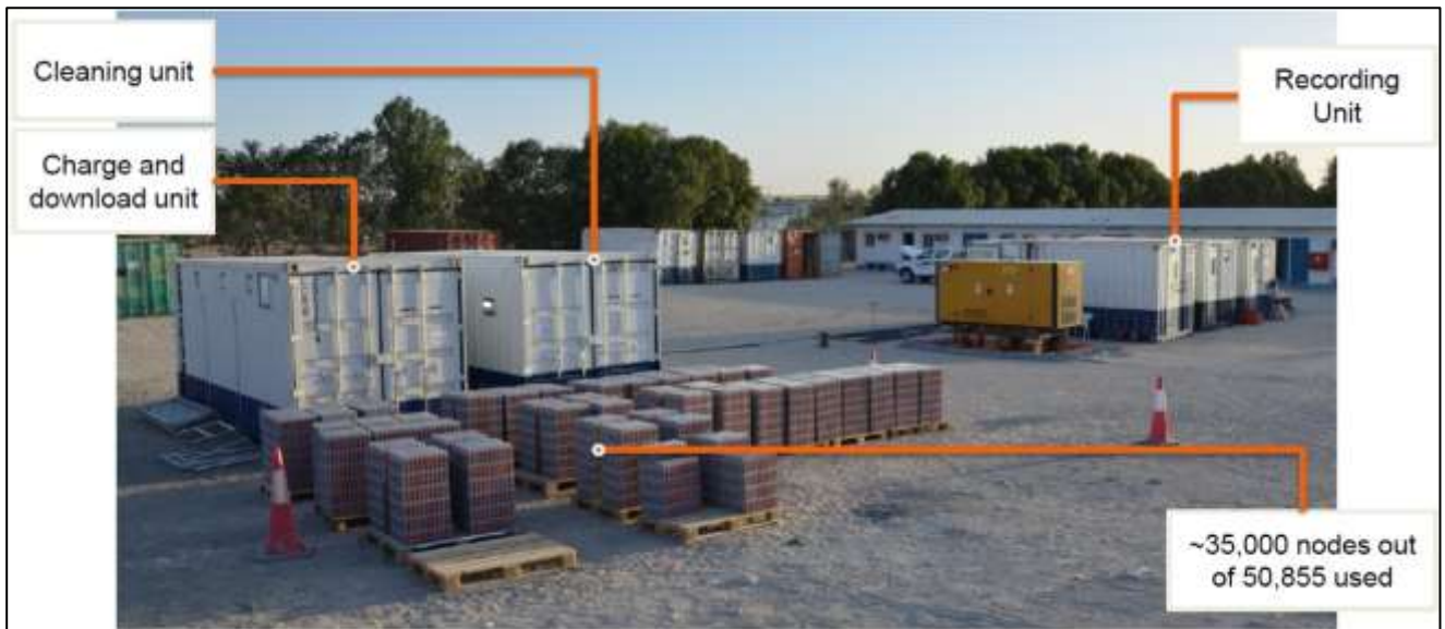
Plate 2.3: Exaple of the conaterised field-based data processing facility and supporting services that will be avaiable for the entire durataion of the proposed 2D seimsic survey operations (Source: www.polarisexplorer.com ).
