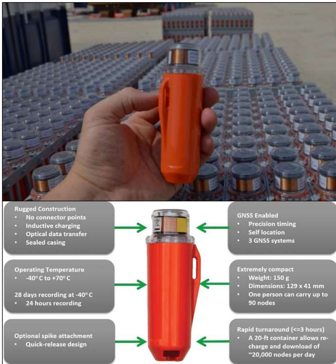
Plate 2.2: The STRYDE wireless recording instrumentation is the latest technology to be used for the proposed 2D seismic survey operations.
