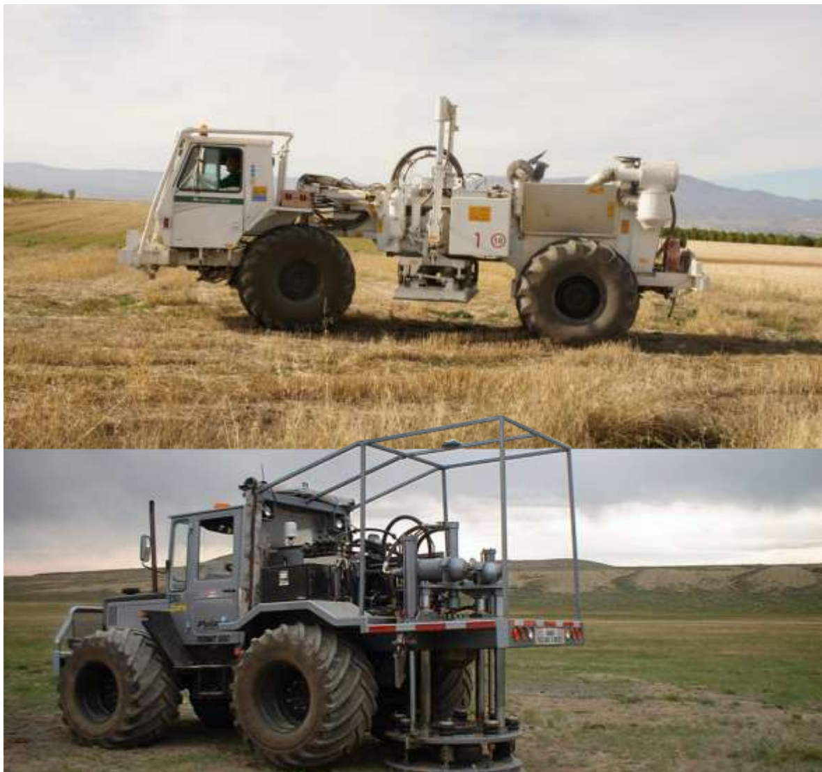
Plate 2.1: Size comparative of the Vibroseis truck (top) and Explorer 860 Accelerated Weight Drop (AWD) (bottom) (Sources: www.polarisexplorer.com ).
